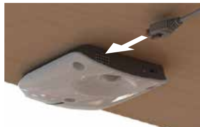
FIG. 6: PLUG MINIFIT INTO LOGICLINK
