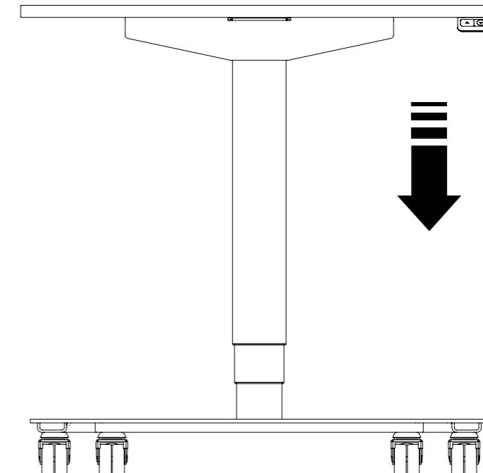
Lower the frame to its lowest position by pressing the down arrow on the hand control. Release the button. Press the button again and keep it pressed for 10 seconds, the reset is now carried out and the frame is ready to use.
