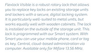
A lock for easier storage. Flexlock Visible is fitted externally and can be installed on units made from both wood and metal. It is compatible with the majority of storage units and lockers that are currently equipped with cylinder locks with 19 mm and 22 mm diameters. The lock is battery powered and no external power supply is required. The LED on the lock flashes green if the unit is free.
